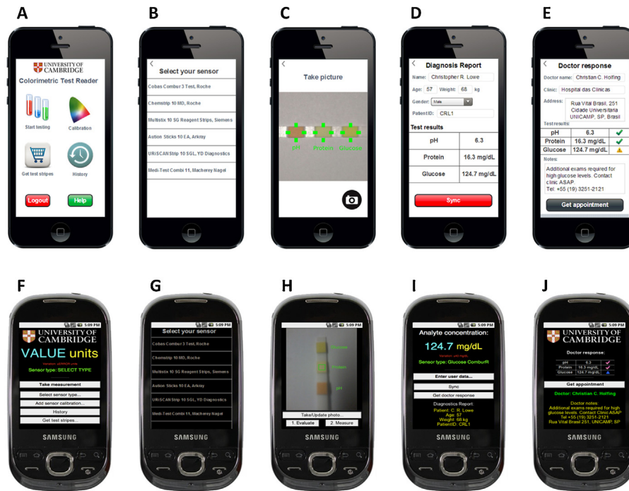
Fig. 2. Screenshots of the iOS and Android apps used to quantify a colorimetric test. (A) Main menu displaying sample testing, calibration and test history viewing. (B) The app displays sensor types. (C) User captures the image of the test zones. (D) The diagnostic test results are displayed to the user. (E) The information received from the physician displayed on the final screen may include user-specific instructions. (F–J) Android version of the same steps A–E, respectively.
